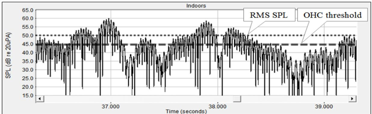
Figure 7 - 22.9 Hz tone fluctuation and OHC threshold
